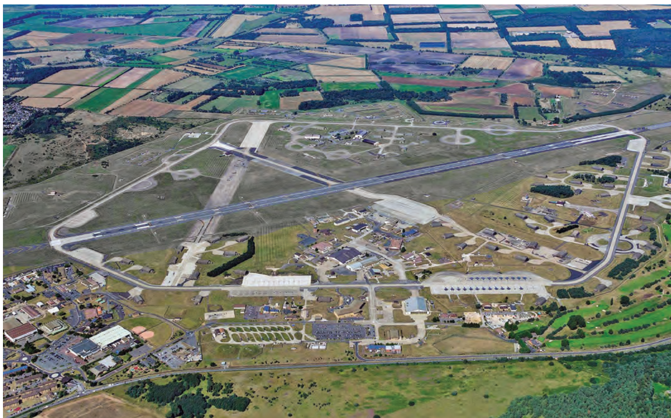
Aerial shot of RAF Lakenheath. The domestic site is to the left, the operational runway runs left to right. Beneath this are the three squadron areas with their Hardened Aircraft Shelters and the technical area (centre)
